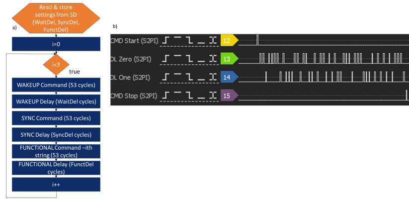
Figure 3: FSM for the Downlink interface and four-wire interface example.
